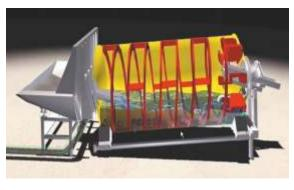
water through the drum overflow. Flushing water for the washing drum can be drawn directly from the slurry tank using a centrifugal water pump. The overfill warning for the washing drum is released by measuring the power consumption of the drive motors and automatic switch on/off control of the feed hopper vibrators. This safety feature is possible with the free feed system used in the Stetter washing drum.
