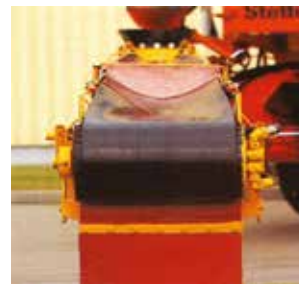
110° belt trough angle for reliable and clean material conveyance
