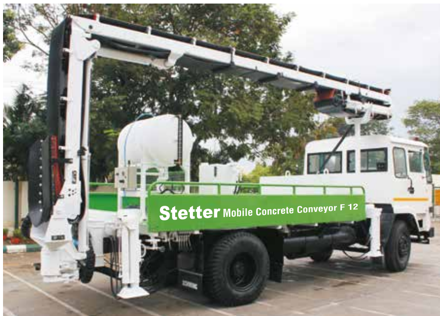
Outriggers at front and rear to provide support
