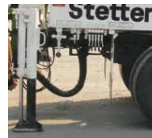
Outriggers at front and rear to provide support
