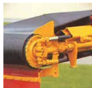
The compacted belt drive permits unimpeded work in confined spaces.
