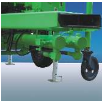
Maintenance free hydraulic cylinder
